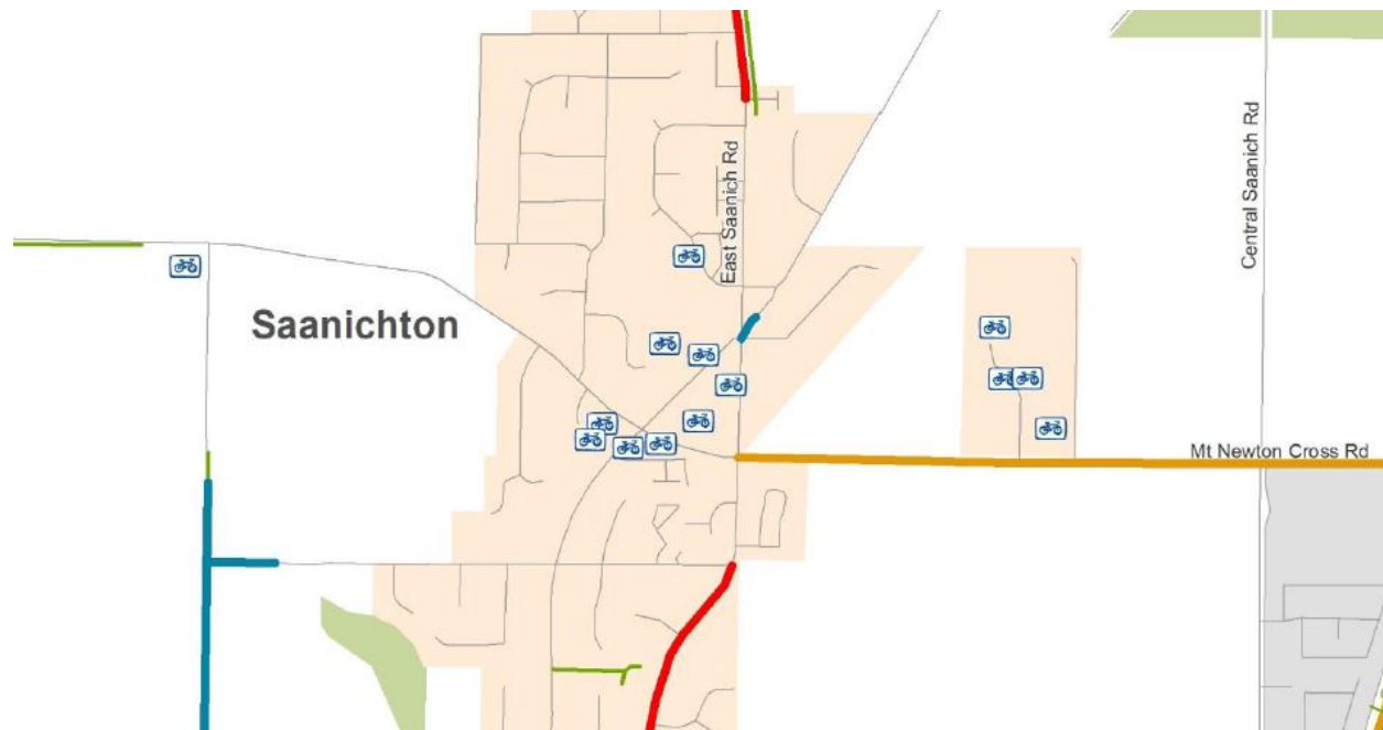
Figure 18. Example of Bike Network Connectivity Gaps in Saanichton, where red indicates a bike lane, green indicates a local trail, orange indicates a shoulder bikeway, blue indicates a shared trail, and bike icons represent bike racks.
